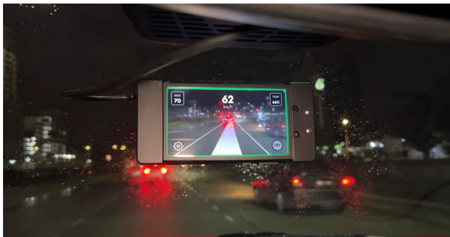
Figure 4: The Advance Driver Assistance System (ADAS) Of the Kommuassist
